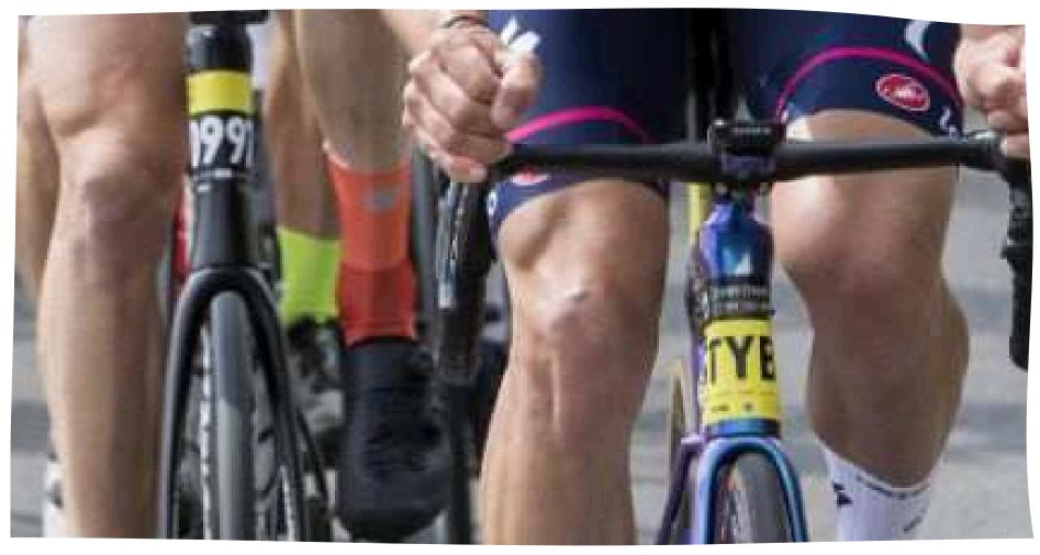
possible way of attaching the start number if you have an integrated/aero cockpit
